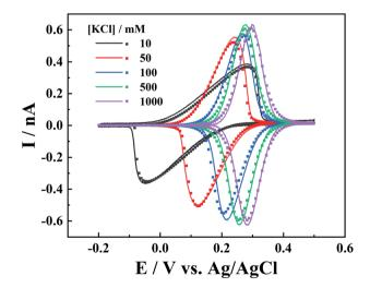
Fig. 5 Experimental (solid lines) and simulated (points) i-V curves for different concentrations of KCl ( $c_1$ ). The K<sub>4</sub>Fe(CN)<sub>6</sub> concentration is 1 mM.  $c_1$ , mM: 10, 50, 100, 500, and 1000. a=50 nm, d=1100a, tan  $\theta=0.19$ , v=0.1 V s<sup>-1</sup> and  $E_0$  is 0.12, 0.18, 0.24, 0.265, and 0.29 V.
