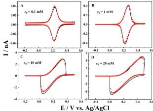
Fig. 4 Experimental (black solid lines) and simulated (red points) i–V curves for different concentrations of K<sub>4</sub>Fe(CN)<sub>6</sub> (c<sub>0</sub>). The background solution is 0.1 M KCl. a = 50 nm, d = 1000a,  $\tan \theta$  = 0.2, v = 0.1 V s<sup>-1</sup> and E<sub>0</sub> = 0.21 V, 0.24 V, 0.2 V, and 0.25 V.
