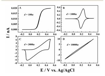
Fig. 3 Simulated i-V responses from a CNP at different solution depths in 1 mM K<sub>4</sub>Fe(CN)<sub>6</sub> + 0.1 M KCl. From panels (A) to (D), the solution depth is 100a, 1000a, 3000a, and 10 000a. a=50 nm,  $\tan\theta=0.2, \ V=0.1 \ {\rm V\ s^{-1}}$  and  $E^0=0.2 \ {\rm V\ }$ .
