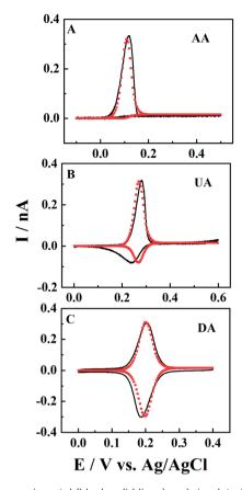
Fig. 7 The experimental (black solid lines) and simulated (red points) voltammograms of AA, UA and DA in CNPs. The concentration is 0.5 mM with 10 mM PBS (pH 7.4) buffer. Fitted value: a=50 nm, d=800a,  $\tan\theta=0.15$ , and v=0.1 V s<sup>-1</sup>.  $k_{\rm c}>0.8$ ,  $k_{\rm c}=0.2$ , and  $k_{\rm c}<0.01$  s<sup>-1</sup> and  $E_0=0.11/0.27/0.2$  V for AA, UA and DA.
