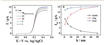
Fig. 1 The simulated steady-state voltammograms of CNPs with different thicknesses (h) of deposited carbon. The solution is 1 mM  $K_4Fe(CN)_6 + 0.1 \text{ M KCl. } a = (50 - h) \text{ nm, } d = 400a, \tan \theta = 0.2, v = 0.1 \text{ V}$  $s^{-1}$  and  $E^{0} = 0.2 \text{ V } vs. \text{ Ag/AgCl.}$
