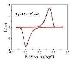
Fig. 6 The cyclic voltammograms of 1 mM FeCl<sub>3</sub> in 0.5 M H<sub>2</sub>SO<sub>4</sub> and 0.1 M KCl from the simulation (red points) and experiments (black solid line). a=100 nm. d=1320a,  $\tan\theta=0.2$ , v=0.1 V s<sup>-1</sup>,  $E_0=0.26$  V and  $k_0=1.3\times10^{-5}$  cm s<sup>-1</sup>.
