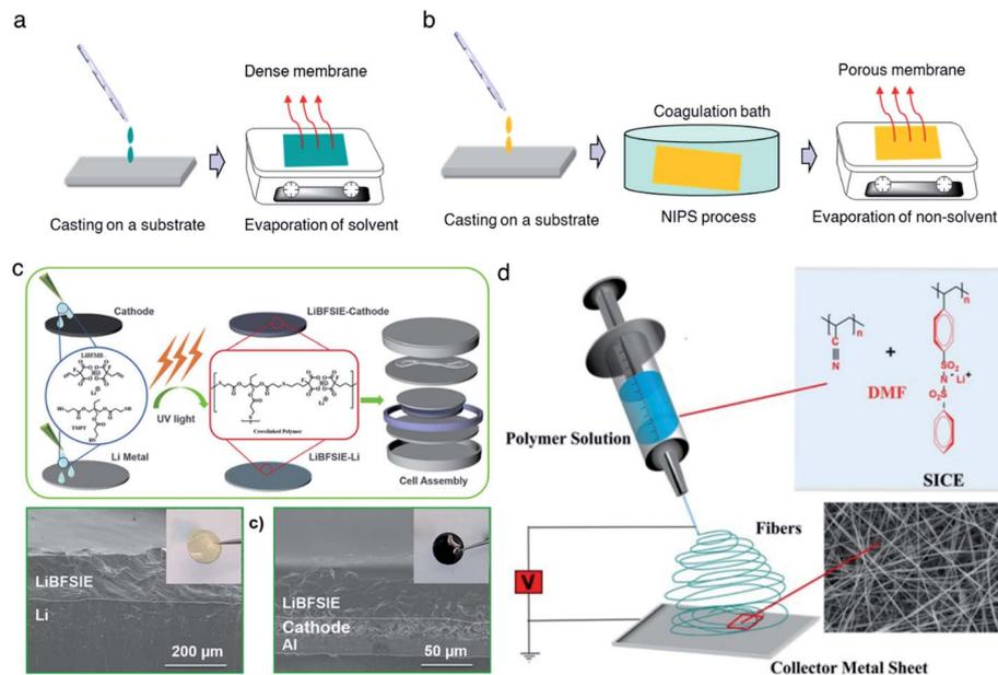
Fig. 9 Schematic illustration of membrane fabrication methods. (a) Casting method. (b) NIPS phase separation. (c) *In situ* polymerization. Reproduced with permission.<sup>94</sup> Copyright 2020, American Chemical Society. (d) Electrospinning technique. Reproduced with permission.<sup>96</sup> Copyright 2017 Wiley.
