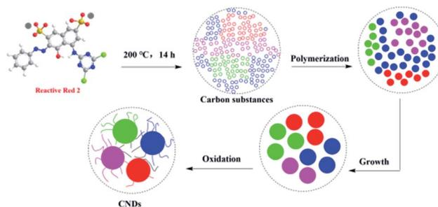
Fig. 6 Proposed mechanism of CNDs formation from RR2.
