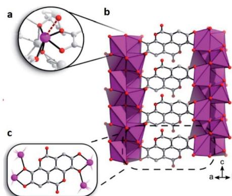
Fig. 12 (a) The coordination environment around Bi<sup>3+</sup>. The bond to a coordinated water molecule is represented as a dashed line. (b and c) Chelation of ellaginate ligand toward the bismuth oxo rods. Reprinted (adapted) with permission from ref. 74. Copyright (2020) American Chemical Society.
