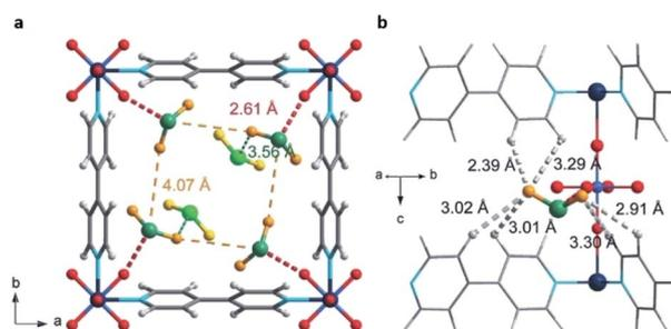
Fig. 7 Binding sites for SO<sub>2</sub> molecules adsorbed within SIFSIX-1-Cu determined by DFT-D calculations. Interaction S<sup>δ+</sup>...F<sup>δ-</sup> (a), and dipole-dipole interactions with the ligand O<sup>δ-</sup>...H<sup>δ+</sup> (b). Cu (dark teal); F (red); Si (light blue); C (grey); H (light grey); N (sky blue); O (orange); S (sea green). Reprinted (adapted) with permission from ref. 51. Copyright (2017) John Wiley & Sons.
