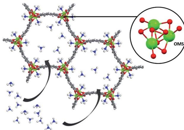
Fig. 18 Atomic structure of  $\text{M}_2(\text{dobpdc})$  complexes with one-dimensional hexagonal channels. It is possible to observe that each coordinatively unsaturated metal site points towards the channel. Reprinted (adapted) with permission from ref. 109. Copyright (2020) John Wiley & Sons.
