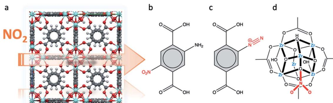
Fig. 23 (a) Structure of UiO-66 analogues. Post functionalization of phenyl ring modifications upon NO<sub>2</sub> sorption: (b) nitration of the phenyl ring, (c) diazonium ion formation. (d) Nitration of the bridging hydroxyl group at the SBU. Reprinted (adapted) with permission from ref. 123. Copyright (2016) John Wiley & Sons.
