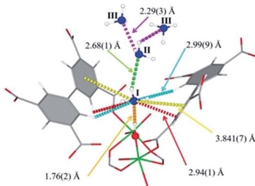
Fig. 19 Binding sites for ND<sub>3</sub> molecules adsorbed within MFM-300(Al) determined by *in situ* NPD studies. Reprinted with permission from ref. 110. Copyright (2018) John Wiley & Sons.
