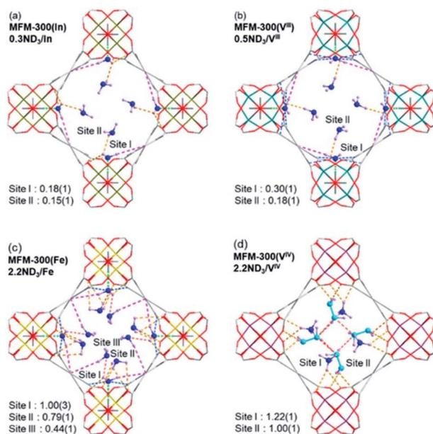
Fig. 20 Preferred ND<sub>3</sub> binding sites in MFM-300(M) family (M = Cr, Fe, V<sup>3+</sup>, V<sup>4+</sup>) determined by NPD at 10 K. Views along *c* axis. Reprinted with permission from ref. 111. Copyright (2021) American Chemical Society.
