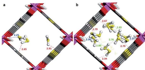
Fig. 10 Illustrative arrangements of H<sub>2</sub>S in the pores of MIL-53-TDC generated from the GCMC simulations at (a) 0.5 mmol g<sup>-1</sup> and (b) 18.5 mmol g<sup>-1</sup>. The distances are reported in Å. (Al, pink; O, red; S, yellow; C, grey; H, white). Reprinted (adapted) with permission from ref. 69. Published (2019) by The Royal Society of Chemistry.
