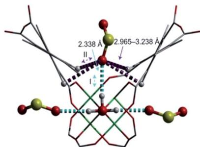
Fig. 2 Preferred binding sites for  $\text{SO}_2$  molecules inside MFM-300(Al) determined by *in situ* PXRD. (I) Moderated hydrogen bond. (II) Weak hydrogen bond. Reprinted (adapted) with permission from ref. 37a. Copyright (2012) Springer Nature.
