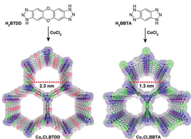
Fig. 17 Structure of  $\text{Co}_2\text{Cl}_2$  BTDD (left) and  $\text{Co}_2\text{Cl}_2$  BBTA (right). C, gray; O, red; N, blue; Cl, green; Co, purple. Hydrogen atoms have been omitted for clarity. Reprinted with permission from ref. 108. Copyright (2018) American Chemical Society.
