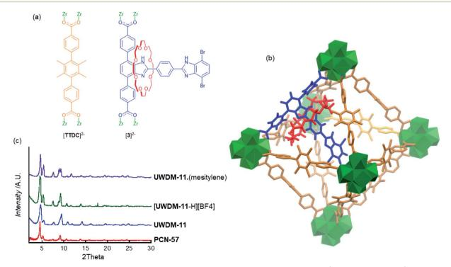
Fig. 3 (a) The two linkers used to construct the multivariate MOF UWDM-11; primary linker [TTDC]<sup>2-</sup> and [2]rotaxane [3]<sup>2-</sup>. (b) A Molecular Studio (Forcite) geometry-optimised model of the octahedral cavity in UWDM-11; MIM axle = blue, 24C8 macrocycle = red, primary [TTDC]<sup>2-</sup> linkers = orange and  $[Zr_6O_4(OH)_4]^{12+}$  nodes = green. (c) PXRD of PCN-57 and various versions of UWDM-11.
