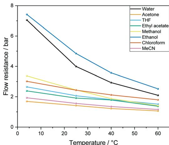
Fig. 5 Calculated overall flow resistance (pressure drop) from 12.4 m PEEK tubing as detailed in Fig. 4 caused by a range of solvents at different temperatures at a flow rate of 4 mL min<sup>-1</sup> according to eqn (1).
