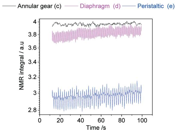
Fig. 21 Absolute  $^1\text{H}$  NMR integral values of acetone flowing through the setup shown in Fig. 12 at a nominal flow rate of  $2 \text{ mL min}^{-1}$  at room temperature using different PD pumps.
