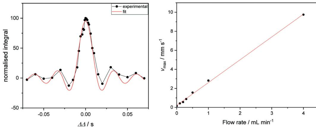
**Fig. 8** Left: Signal intensity as a function of  $\Delta\Delta$  for a flowrate of  $1.0 \text{ mL min}^{-1}$  (see ESI† for graphs of other flow rates). Curve fitting gives access to the maximum velocity. Right: Correlation of linear sample velocities derived from  $\Delta\Delta$  fitting with volumetric flow rates supplied by the peristaltic pump.
