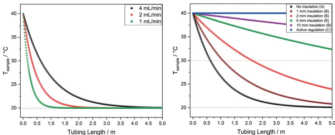
**Fig. 11** Left: Modelled temperature profiles of water at 40 °C flowing through 1.6 mm OD/0.76 mm ID PEEK tubing in air at 20 °C (blue dotted line) at various flow rates, corresponding to scenario A in Fig. 9. Right: Modelled temperature profiles of water at 40 °C flowing through 1.6 mm OD/0.76 mm ID PEEK tubing in air at 20 °C (blue dotted line) at 4 mL min<sup>-1</sup> with different levels of insulation, comparing scenarios A, B and C from Fig. 9.
