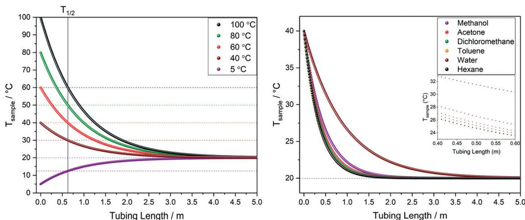
**Fig. 10** Left: Modelled temperature profile of water over tubing length at different starting temperatures. Right: Comparison of temperature profiles for different solvents starting at 40 °C. All at 4 mL min<sup>-1</sup> flow rate through 1.6 mm OD/0.76 mm ID PEEK tubing in air at 20 °C (blue dotted line) corresponding to scenario A in Fig. 9.
