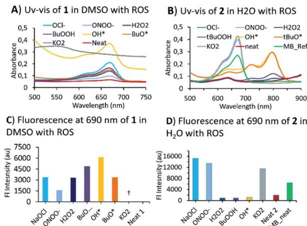
Fig. 2 Optical properties of MB-BHT ( $25 \text{ nmol mL}^{-1}$ ) after treating sufficient amount of ROS ( $>5$  equiv.). Fluorescence emission (concentration  $12 \text{ nmol mL}^{-1}$ ) at the maximum of  $689 \text{ nm}$  for excitation at  $645 \text{ nm}$  ( $\ddagger$ : due to fast decomposition of the formed MB).
