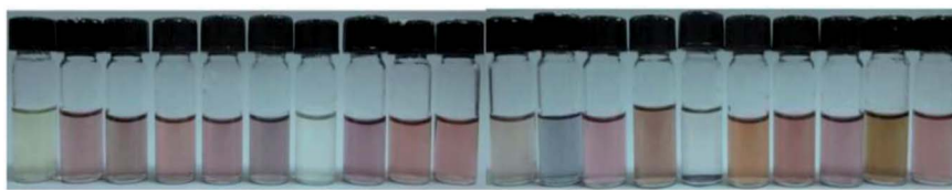
Fig. 7 Optical images of the final GNs solution of AAFGQDs in daylight (from left to right: Cys, Ala, Asp, Glu, Phe, Gly, His, Ile, Lys, Leu, Met, Asn, Pro, Gln, Arg, Ser, Thr, Val, Trp, and Tyr). The figure has been reproduced from ref. 93 with permission from Royal Society of Chemistry, copyright 2016.
