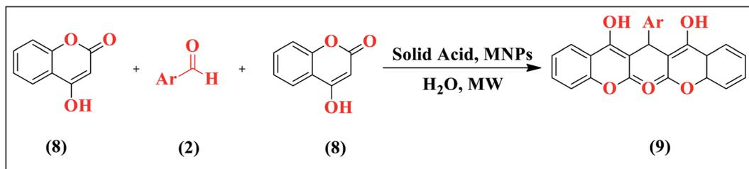
Scheme 3 Synthesis of bis-coumarin derivatives in Fe<sub>3</sub>O<sub>4</sub>@sulfosalicylic acid MNPs as catalyst under microwave irradiation in water.
