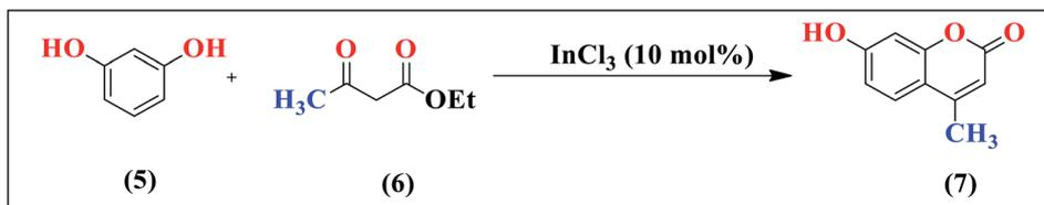
Scheme 29 Synthesis of coumarins via von Pechmann condensation of phenols with  $\beta$ -ketoesters induced by  $\text{In}(\text{III})\text{Cl}_3$ .
