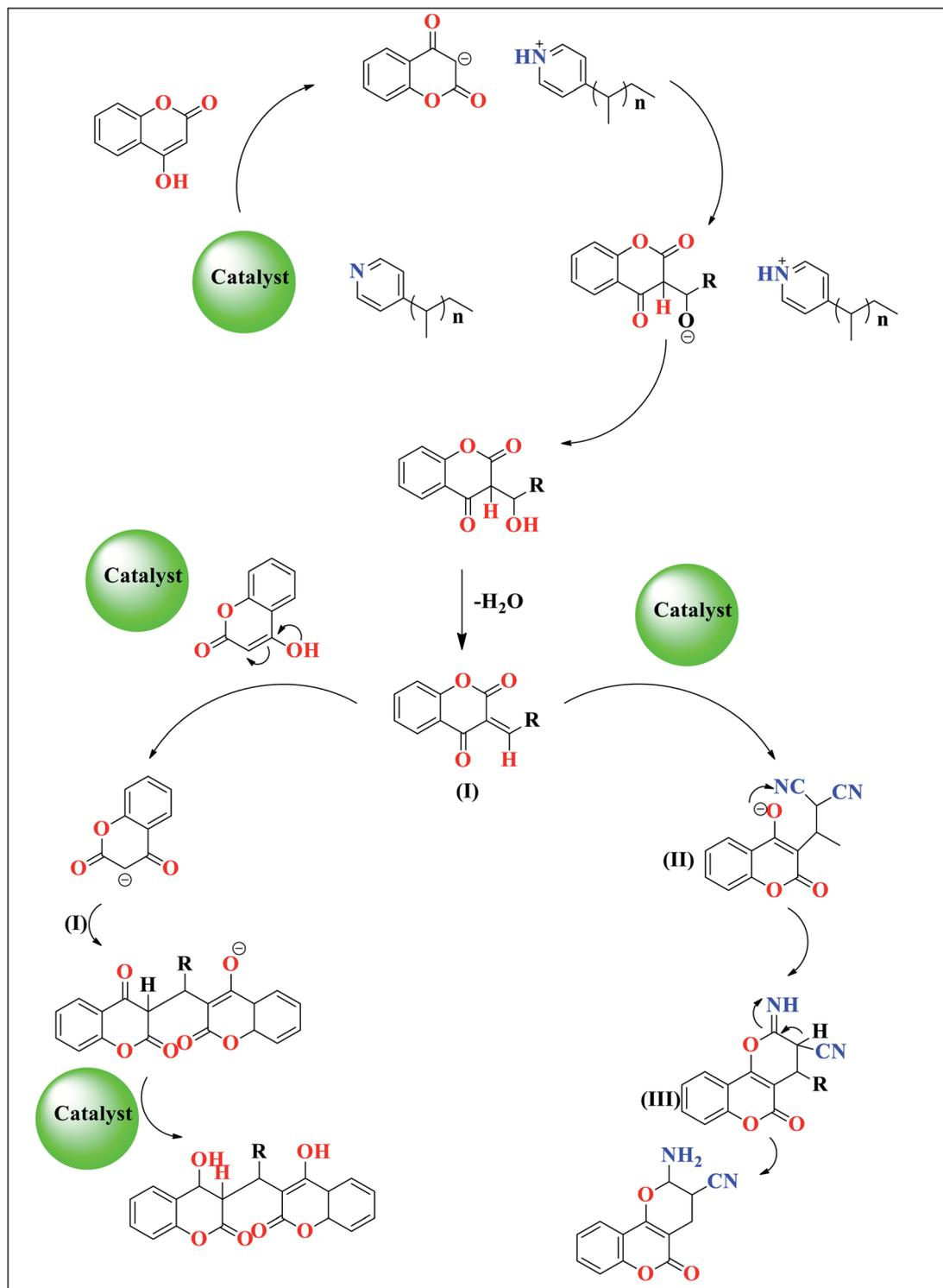
Fig. 6 Proposed mechanism for the synthesis of dihydropyrano[3,2-c]chromene and biscoumarin derivatives in the presence of P<sub>4</sub>VPy as catalyst.
