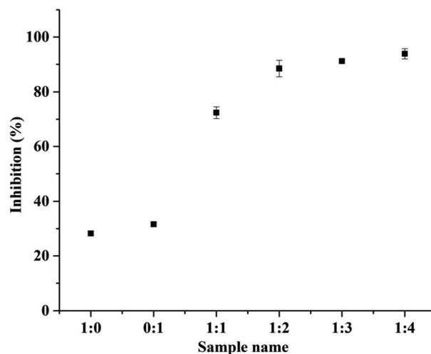
Fig. 6 DPPH radical scavenging activity of controls BSA (1 : 0), dextran (0 : 1) and BSA–dextran conjugates of molar ratio 1 : 1, 1 : 2, 1 : 3 and 1 : 4. Data represent mean values  $\pm$  SE of three independent experiments performed in triplicates.
