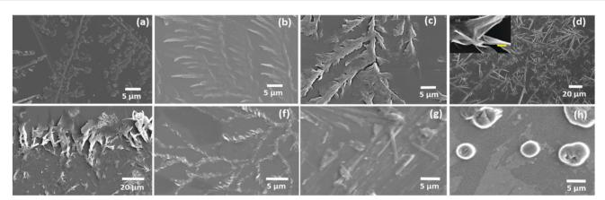
Fig. 1 FE-SEM images of Gly (a), Ala (b), Leu (c), Ile (d), Val (e), Met (f), Pro (g) displaying the formation of microcrystals arranged in fern-like architectures, and Cys (h) displaying the formation of globular structures [ESI,† Table S2 for specific set of conditions].
