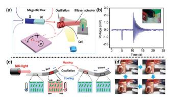
Fig. 16 (a) Schematic illustration of the mini-generator based on the UV-responsive bending motion; adapted with permission from ref. 95. Copyright 2015 American Chemical Society. (b) Induced voltage of the mini-generator; (c) mechanism of the NIR-light-driven oscillation motion of the NIR-responsive film; (d) apparatus of the NIR-driven mini-generator. Adapted with permission from ref. 96. Copyright 2020 Wiley.
