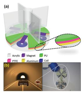
Fig. 21 (a) Structural design of the wind-driven hybridized mini-generator; (b) schematic illustration of harvesting wind energy in the tunnel and the photograph of the mini-generator. Adapted with permission from ref. 104. Copyright 2016 American Chemical Society.
