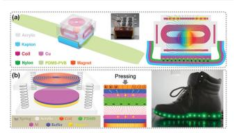
Fig. 20 (a) Schematic illustration of the fabrication and the working principle of the watch-like hybridized mini-generator; adapted with permission from ref. 101. Copyright 2015 American Chemical Society. (b) Function mechanism of the mini-generator when embedded into shoes during human walking. Adapted with permission from ref. 102. Copyright 2015 American Chemical Society.
