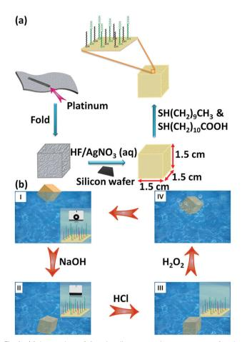
Fig. 1 (a) Integration of functionally cooperative components for the fabrication of a self-propulsive device; (b) the cycled diving-surfacing movement realized via cooperation between the components. Adapted with permission from ref. 16. Copyright 2010 Wiley.
