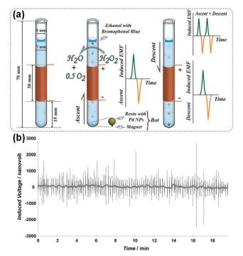
Fig. 6 (a) The surfacing/diving vertical motion of the micro bot in a glass tube. Each surfacing/diving motion generates an EMF signal as shown in the plots beside the tubes; (b) induced voltage generated from the motion of the micro bot. Adapted with permission from ref. 18. Copyright 2014 Wiley
