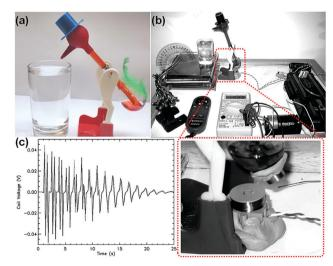
Fig. 10 Photographs of (a) a drinking bird and (b) the experimental setup of the mini-generator based on a drinking bird; (c) the induced voltagetime curve. Adapted with permission from ref. 37, Copyright 2006 AIP Publishing; from ref. 38, Copyright 2019 Scientific Research Publishing Inc.
