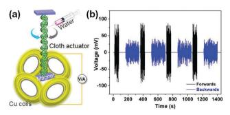
Fig. 13 (a) Schematic illustration of mini-generators based on hygroscopic cloth actuator; (b) induced voltage up to 75 mV produced by the mini-generator. Adapted with permission from ref. 97. Copyright 2017 Wiley.
