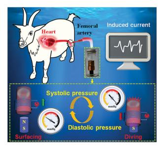
Fig. 17 Schematic illustration of the blood pressure-responsive minigenerator system. Adapted with permission from ref. 36. Copyright 2019
