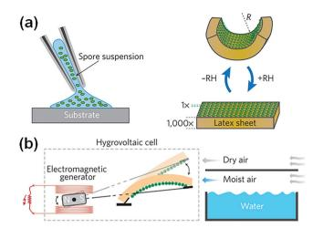
Fig. 14 (a) Schematic illustration of the assembly of the spore on a latex sheet and the bending motion of the actuator; (b) apparatus of the minigenerator based on the spore actuator. Adapted with permission from ref. 93. Copyright 2014 Springer Nature.
