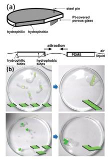
Fig. 25 (a) Design of PDMS plates for self-propulsion and assembly via capillary attraction. Adapted with permission from ref. 65. Copyright 2002 Wiley. (b) MSA patterns of line or triangle structures directed by anisotropic modification. Adapted with permission from ref. 32. Copyright 2014 Wiley.
