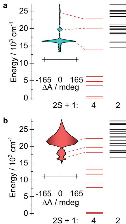
**Fig. 6** (a) MCD spectra of compound **1** obtained at 1.55 K with an applied field of +7 and -7 T (see Fig. S18†). The calculated doublet and quartet electronic state are represented by black and red lines, respectively. (b) The corresponding data are shown for compound **3**.
