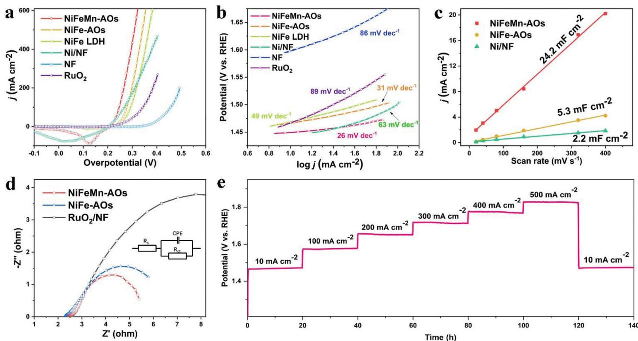
Fig. 3 The performance of the oxygen evolution reaction. (a) The LSV curves of various electrodes. (b) The Tafel plots calculated from polarization curves. (c) C<sub>dl</sub> values of Ni/NF, NiFe-AOs and NiFeMn-AOs. (d) EIS Nyquist plots of RuO<sub>2</sub>/NF, NiFe-AOs and NiFeMn-AOs electrodes with 250 mV overpotential. (e) Multi-chronopotentiometry curves of NiFeMn-AOs under various current densities.
