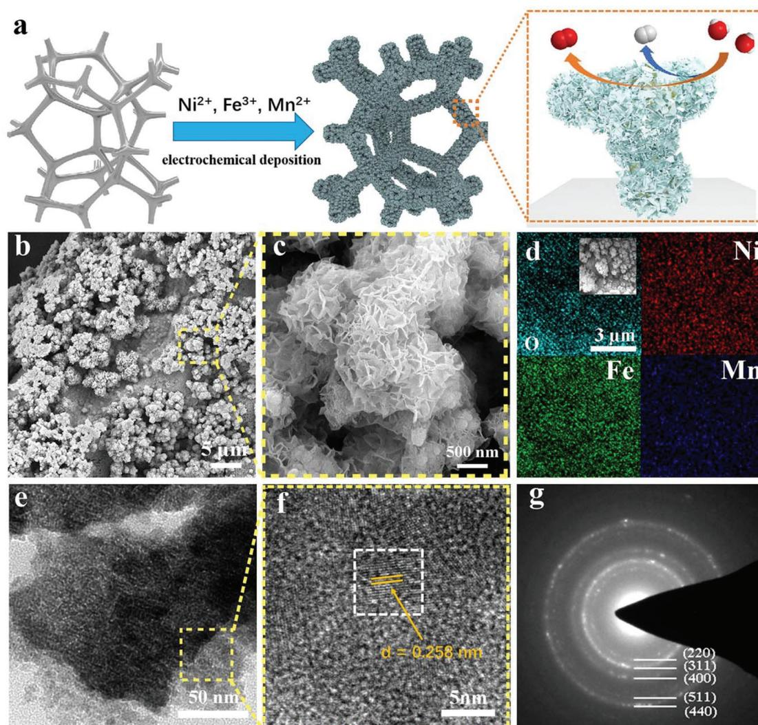
**Fig. 1** (a) Schematic illustration of the fabricating process of the NiFeMn-AOs electrode and its catalytic function for both OER and HER. (b and c) SEM images of the NiFeMn-AOs at different magnification. (d) EDX elemental mapping images from SEM. (e) Scanning TEM image of the NiFeMn-AOs. (f and g) HRTEM image of NiFeMn-AOs and corresponding SAED.
