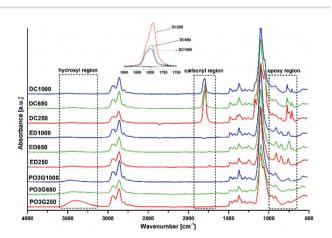
**Fig. 2** FTIR spectra of the original bio-based polyether polyols (PO3G250, PO3G650 and PO3G1000), the synthesized diglycidyl ethers (ED250, ED650 and ED1000) and the synthesized bis(cyclic carbonate)s (DC250, DC650 and DC1000).
