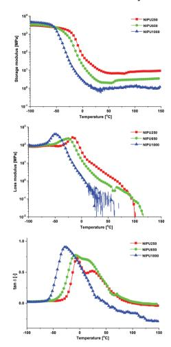
Fig. 10 The DMTA results of NIPU250, NIPU650 and NIPU1000 non-isocyanate polyurethanes synthesized by the ring-opening polyaddition of the DC250, DC650 and DC1000 bis(cyclic carbonate)s, respectively.
