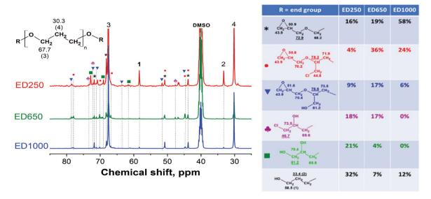
Fig. 5 13C NMR spectra of the synthesized diglycidyl ethers (ED250, ED650 and ED1000), peak denotation and end group characterization and quantification.
