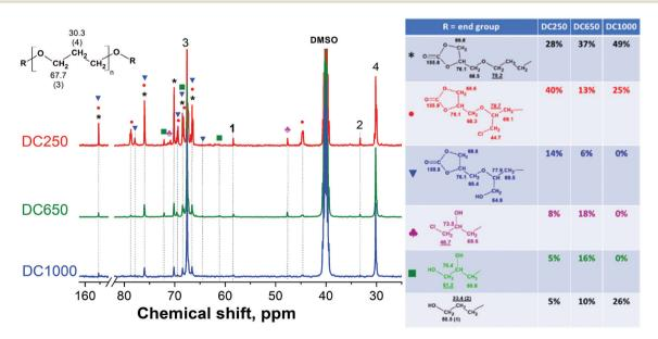
Fig. 6 <sup>13</sup>C NMR spectra of the synthesized bis(cyclic carbonate)s (DC250, DC650 and DC1000), peak denotation and end group characterization and quantification.
