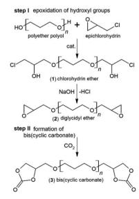
Fig. 1 Scheme of the reaction between polyether polyol and epichlorohydrin (I step) and cycloaddition of CO<sub>2</sub> into diglycidyl ether (II step).
