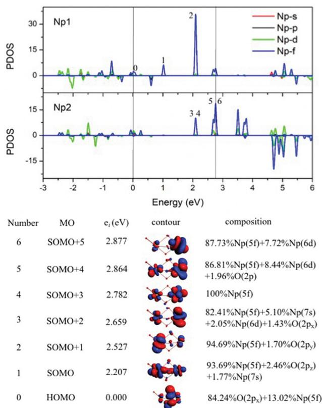
**Fig. 5** Upper occupied canonical Kohn–Sham valence MO envelopes of the septet  $\text{Np}_2\text{O}_4$  molecule. SOMO and SOMO+1 orbitals are distributed more on the Np1 atom while SOMO+2 to SOMO+5 orbitals are distributed more on the Np2 atom. The value of the contour envelopes is 0.02 a.u.
