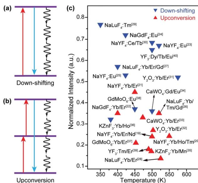
**Fig. 1** Schematic illustration of nonradiative quenching in (a) down-shifting and (b) upconversion luminescence processes. (c) Reported relative emission intensity as a function of temperature in typical inorganic luminescent materials, demonstrating the higher susceptibility of upconversion to thermal quenching than relevant down-shifting luminescence. The emission intensities at the room temperature are set as unity.
