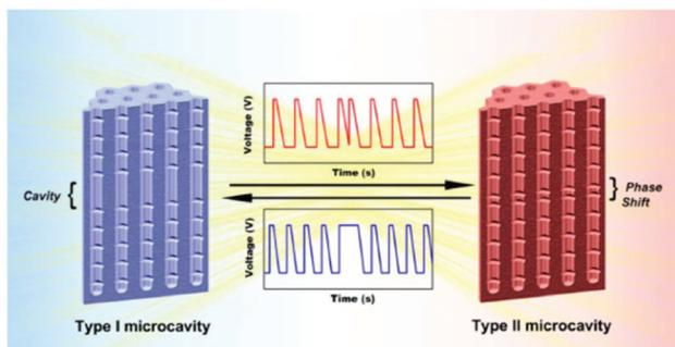
**Fig. 25** Illustration of the fabrication process of AAO microcavities by pulse anodization. Type I microcavities are prepared by inserting a cavity layer between the AAO-DBR structures (left side in blue). Type II microcavities are fabricated by shifting the phase of anodization to achieve the phase modulation of an effective refractive index in the bottom Bragg reflector structure (right side in red). Reprinted with permission from ref. 363. Copyright © 2015, the American Chemical Society.
