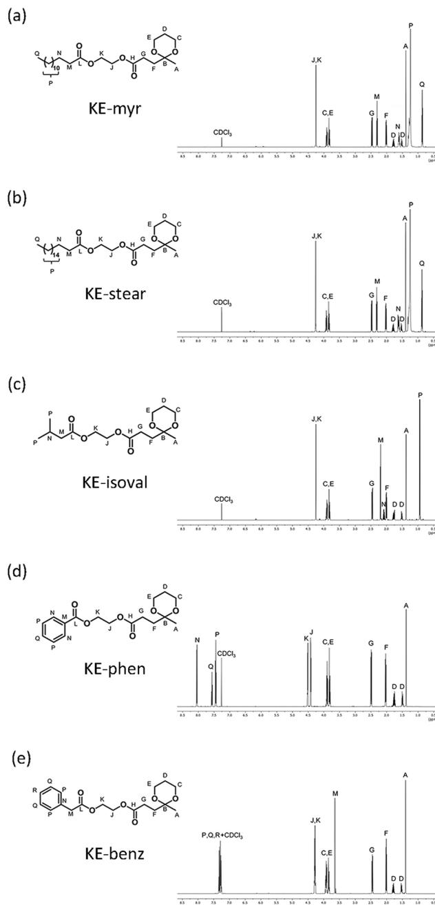
Fig. 1 <sup>1</sup>H-NMR spectra and the corresponding proton assignments of the final ketal-esters: (a) KE-myrr, (b) KE-stear, (c) KE-isoval, (d) KE-phen and (e) KE-benz.
