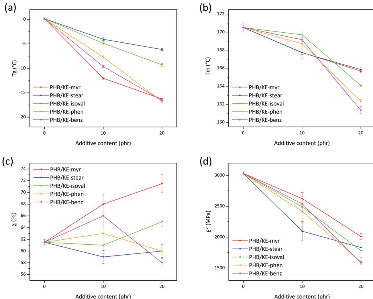
Fig. 4 (a) Glass transition temperature ( $T_g$ ) and (b) melting temperature ( $T_m$ ) determined by DSC for neat and plasticized PHB films as a function of the additive content. (c) Crystallinity degree ( $\chi$ ) calculated using eqn (2) from the DSC curves for neat and plasticized PHB films as a function of the additive content. (d) Storage modulus ( $E'$ ) values (extrapolated at 25 °C) as a function of the additive content for neat and plasticized PHB films.
