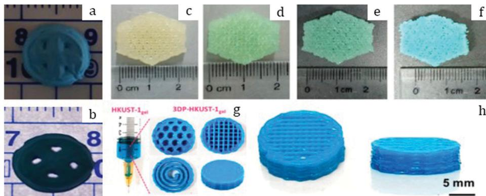
Fig. 12 Photographs of objects 3D-printed *via* the DIW method: CPL-1 before (a) and after drying (b) prepared by Dhainaut *et al.*<sup>115</sup> Copyright 2020 American Chemical Society. Printed objects with HKUST-1 loadings of 0% (c), 2.5% (d), 3.7% (e) and 13% (f) prepared by Pei *et al.*<sup>116</sup> Copyright 2020 Elsevier. HKUST-1 gel in a syringe (g) and monoliths (g and h) prepared by Lim *et al.*<sup>117</sup> Copyright 2019 American Chemical Society.
