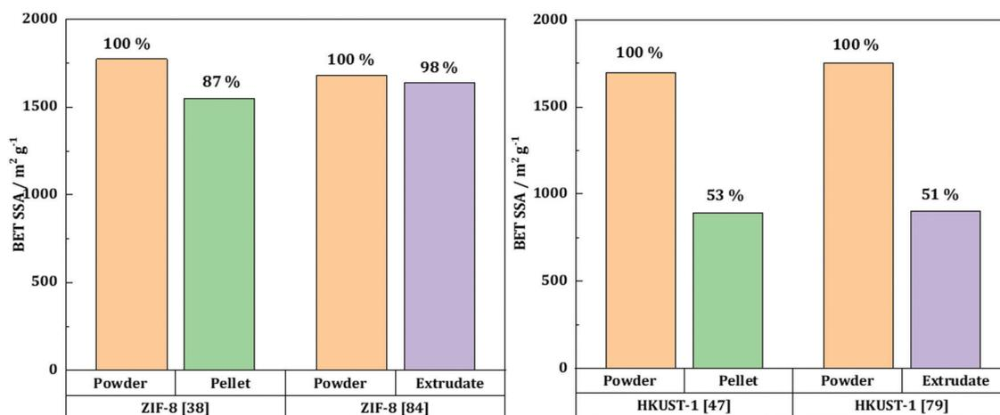
Fig. 8 Comparison of the extruded<sup>84</sup> and pelletized<sup>38</sup> ZIF-8 (left); and the pelletized<sup>47</sup> and extruded<sup>79</sup> HKUST-1 (right). Numbers indicate the BET SSA upon shaping the pristine powder into extrudates and pellets.
