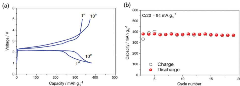
Fig. 18 (a) Voltage profiles and (b) cycling behavior of a Li/Li<sub>2</sub>S–P<sub>2</sub>S<sub>5</sub>/S–MCMB cell. Image reprinted with the permission from ref. 132. Copyright © 2021, Elsevier License 5041400972622.
