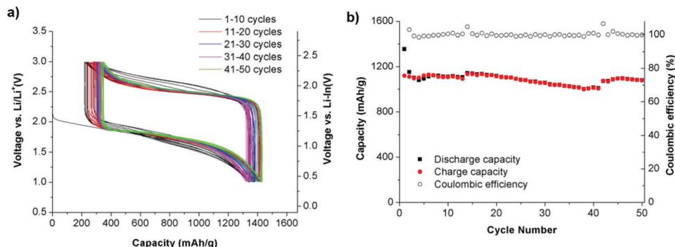
Fig. 20 (a) Discharge-charge curves and (b) discharge/charge capacity and coulombic efficiency of the all-solid-state S/Li<sub>6</sub>PS<sub>5</sub>Br/In-Li cell up to 50 cycles at room temperature. Image reprinted with permission from ref. 134. <https://doi.org/10.1007/s10008-014-2654-1>.
