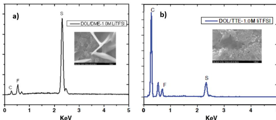
Fig. 29 EDS spectra of the sulfur electrode at the first discharge using (a) 1.0 M LiTFSI DOL/DME and (b) 1.0 M LiTFSI DOL/TTE electrolytes. Image reprinted with the permission from ref. 147. Copyright © 2013, Elsevier License 5041341180684.
