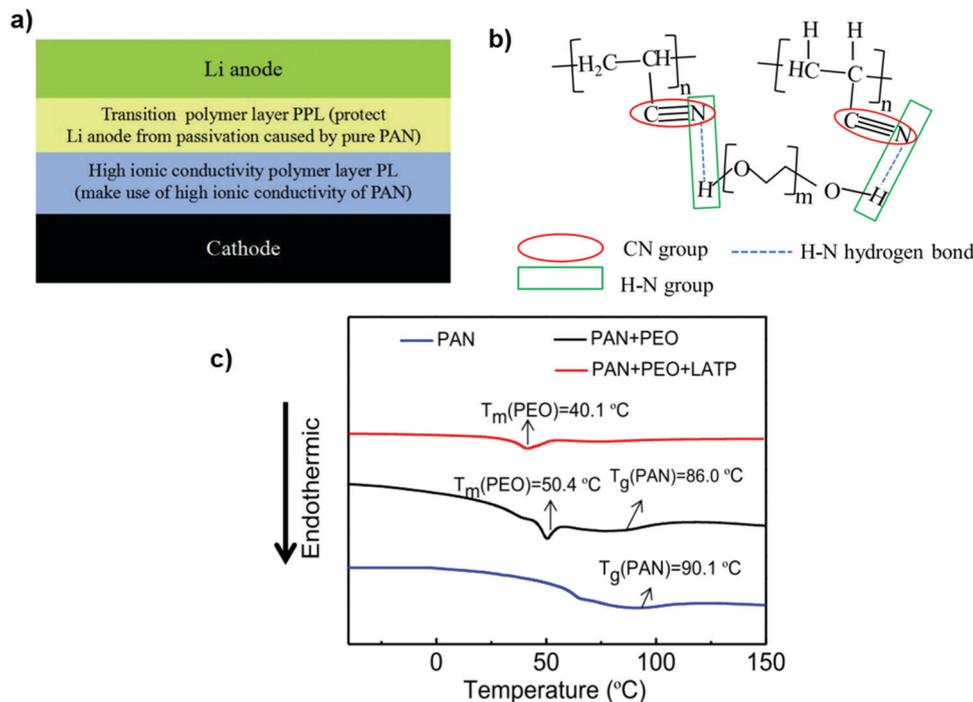
**Fig. 16** (a) Working mechanism and stacking model of the PPL-PL electrolyte. (b) Schematic diagram of the intermolecular hydrogen-bonding effect between PAN and PEO and the passivation-weakening mechanism of CN groups by hydrogen bonds. (c) DSC curves of PAN, PAN + PEO, and PAN + PEO + LATP. Image reprinted with the permission from ref. 108. Copyright © 2019, Elsevier License 5041391264234.
