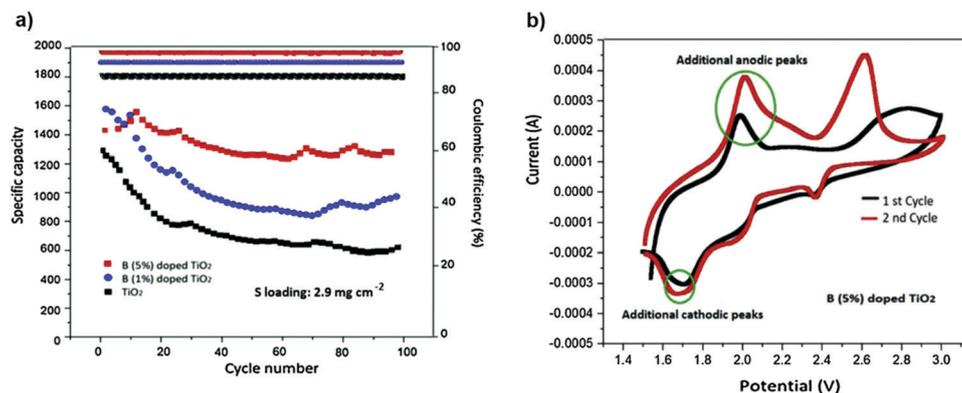
Fig. 26 (a) Cycling performance and coulombic efficiency of Li-S cells for three different coatings at 1 C. (b) First two CV curves of the cell with a 5% B-doped  $\text{TiO}_2$  coating swept at  $0.1 \text{ mV s}^{-1}$ . Image reprinted with the permission from ref. 140. Copyright © 2020, Elsevier License 5040720744337.
