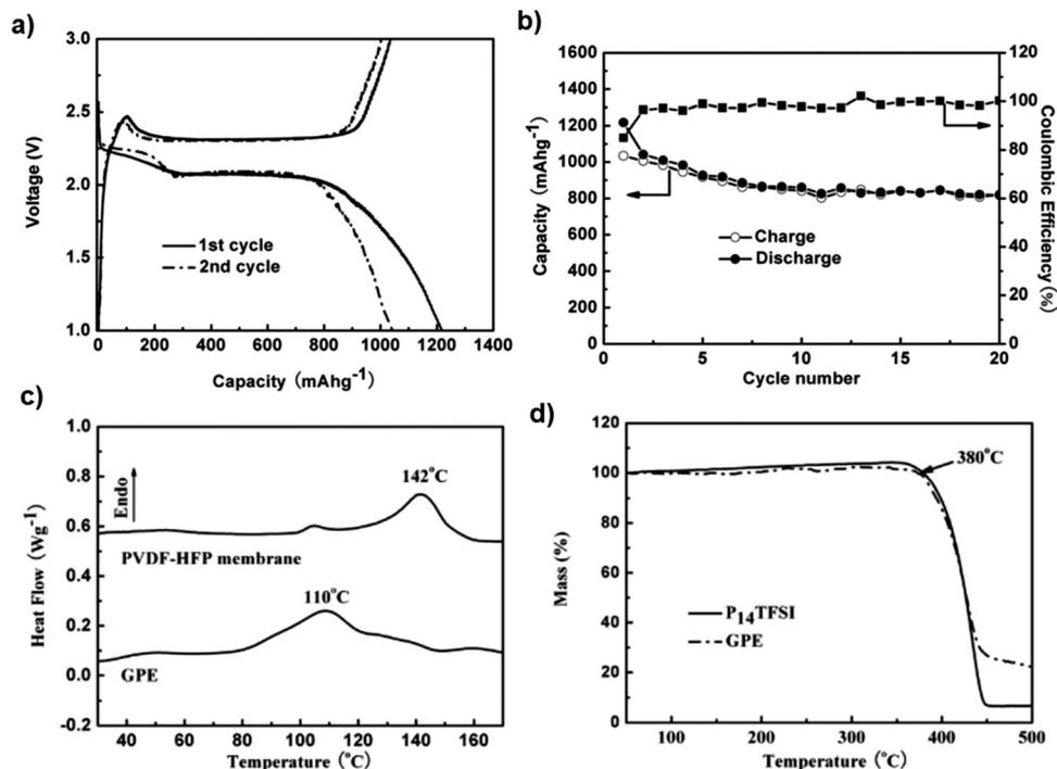
Fig. 12 (a) Charge–discharge curves and (b) cycling performance of the Li/GPE/S battery at a current density of 50 mA g<sup>-1</sup>. (c) DSC curves of P(VDF-HFP) membrane and GPE, and (d) TGA of P<sub>14</sub>TFSI and GPE. Image reprinted with the permission from ref. 104. Copyright © 2012 Elsevier License 5041380226718.
