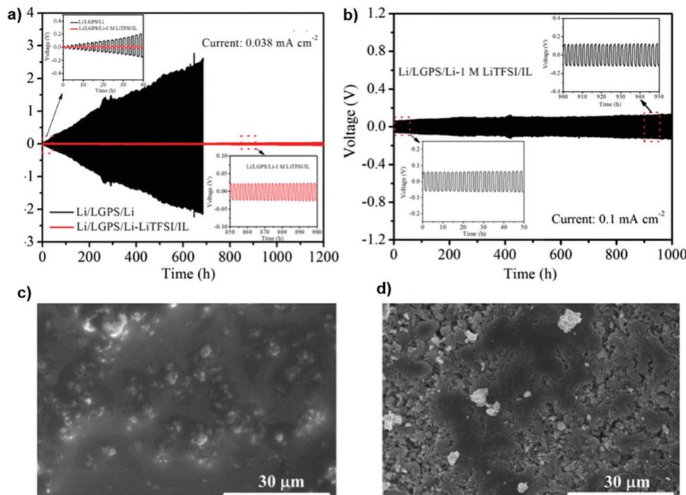
Fig. 21 (a) Galvanostatic cycling curves of cells with and without 1 M LiTFSI/IL at 0.038 mA cm<sup>-2</sup> and (b) the cell with 1 M LiTFSI/IL. SEM images after long-term Li stripping/plating cycles for the cells (c) with and (d) without 1 M LiTFSI/IL. Image reprinted with permission from ref. 135. Copyright © 2019, American Chemical Society.
