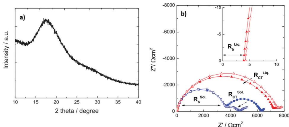
Fig. 19 (a) XRD diffraction pattern of Li<sub>3</sub>PS<sub>4</sub> and (b) Nyquist plots of solid (blue) and liquid (red) electrolyte symmetrical Li/Li cells at  $-20\text{ }^{\circ}\text{C}$ . Image reprinted with the permission from ref. 133. Copyright © 2015 IOP publishing *J. Electrochem. Soc.* <https://doi.org/10.1149/2.0441504jes>.
