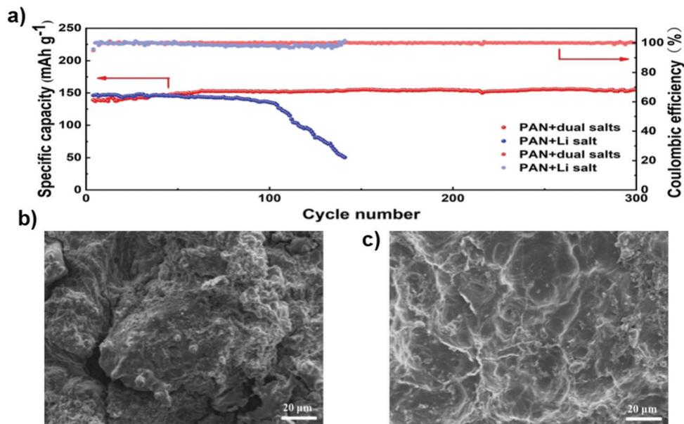
Fig. 24 (a) Long-term cycling performance of cells with different electrolytes at the 0.5 C rate. (b) SEM image of the surface of the metal lithium electrode in cells, without the magnesium salt added to the electrolyte, after 200 cycles, and (c) SEM image of the surface of the metal lithium electrode in the cells, with magnesium salt added to the electrolyte, after 200 cycles. Image reprinted with permission from ref. 138. Copyright © 2020, Royal Society of Chemistry License 1116857-1.
