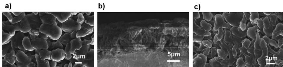
Fig. 22 (a) SEM micrographs of a Li electrode after 10 cycles at  $2 \text{ mA cm}^{-2}$  in LiFSI–LiTFSI/DOL–DME electrolyte. (b) Cross-section micrograph of metallic lithium after 5 cycles in the LiFSI–LiTFSI/DOL–DME electrolyte. (c) SEM micrograph of lithium deposited after 51 cycles in LiFSI–LiTFSI/DOL–DME solution at  $10 \text{ mA cm}^{-2}$ . Image reprinted with permission from ref. 136. Copyright © 2020, Royal Society of Chemistry License 1116857-1.
