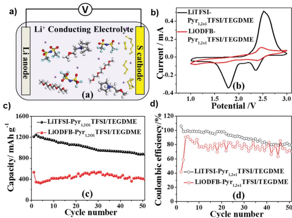
Fig. 23 (a) Schematic illustration of the Pyr<sub>1.201</sub>TFSI/TEGDME electrolyte with LiTFSI. (b) CVs of the Li–S cells containing the Pyr<sub>1.201</sub>TFSI/TEGDME electrolytes with LiTFSI and LiODFB. (c) Cycling performance and (d) coulombic efficiency of the Li–S cells with the LiTFSI–Pyr<sub>1.201</sub>TFSI/TEGDME and LiODFB–Pyr<sub>1.201</sub>TFSI/TEGDME electrolytes. Image reprinted with permission from ref. 137. Copyright © 2015, Elsevier License 5041420221520.
