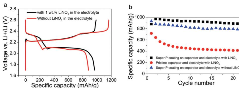
Fig. 25 (a) First charge/discharge voltage profiles of the Li-S batteries using the electrolyte with and without 1 wt%  $\text{LiNO}_3$ , respectively. (b) Cycling stability comparison of the Li-S batteries with different separators and electrolytes at C/10. Image reprinted with the permission from ref. 139. Copyright © 2014, Royal Society of Chemistry License 1116742-1.
