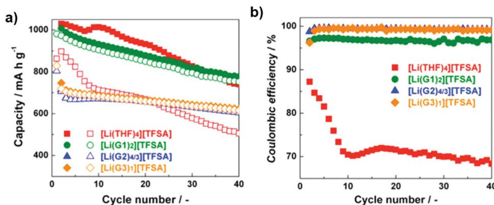
Fig. 8 Cycling performance of Li-S cells with [Li(glyme or THF)<sub>x</sub>][TFSA] (a) capacity; and (b) coulombic efficiency. Image reprinted with the permission from ref. 73. Copyright © 2015, Elsevier License 5041351036896.
