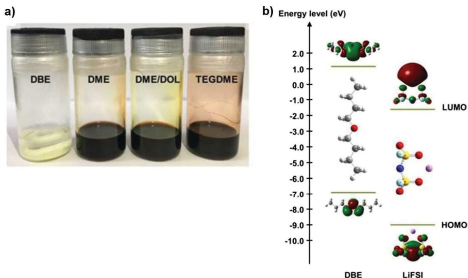
Fig. 4 (a) Photograph of dissolution test of 0.25 M Li<sub>2</sub>S<sub>6</sub> in typical ether solvents by stirring stoichiometric amounts of Li<sub>2</sub>S and sulfur in the solvents for 24 h. (b) The LUMO and HOMO energy values of DBE and LiFSI obtained by DFT simulations. Image reprinted with the permission from ref. 61. Copyright © 2018, Royal Society of Chemistry License-1117493-1.
