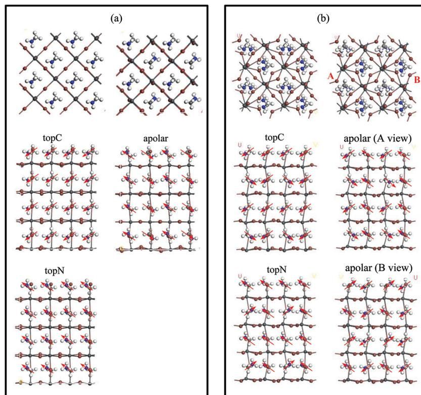
**Fig. 2** Top and side views of (a) cubic and (b) tetragonal MAPbI<sub>3</sub>(001) surfaces with MAI terminations for topC, topN and apolar geometries. Two different side views (from A and B sides) of the tetragonal MAPbI<sub>3</sub>(001) surface are shown for clarity. H, C, N, I, and Pb atoms are represented by the white, light grey, blue, brown, and dark grey spheres, respectively. Red arrow represents the molecular dipole of a MA cation with the NH<sub>3</sub> group as the arrow head.
