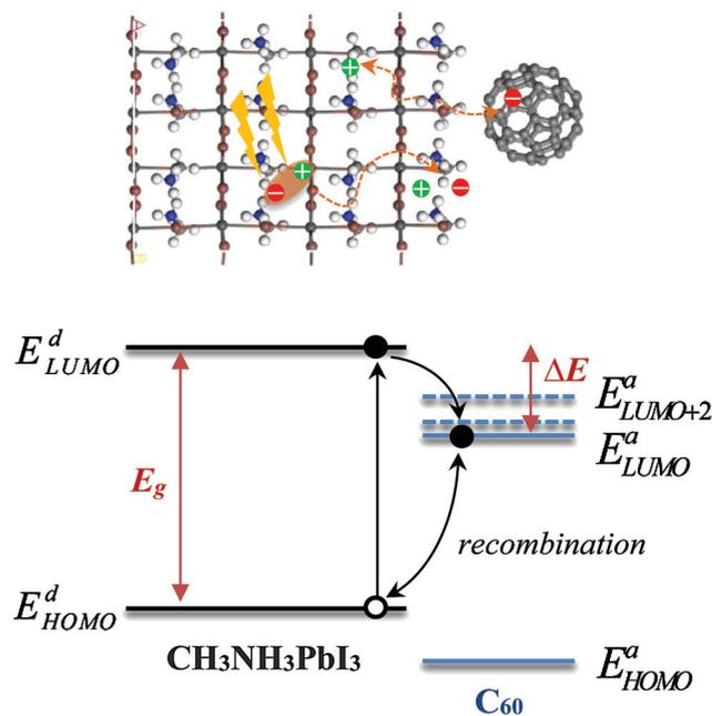
Fig. 1 Schematic illustration of the energy-level diagram for the MAPbI<sub>3</sub> and C<sub>60</sub> in the hybrid perovskite/fullerene heterojunction.  $E_g$  is the energy gap of MAPbI<sub>3</sub> and  $\Delta E$  is the dissociation energy of the electron–hole pairs. The three-fold degenerate LUMO of C<sub>60</sub> fullerene has three energy levels from the LUMO to LUMO+2.
