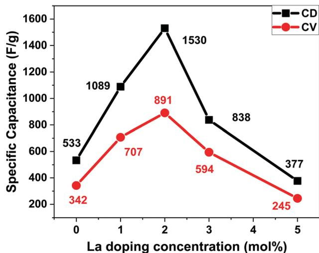
Fig. 10 Specific capacitance vs. doping concentration of La from the CV curve at 5 mV s<sup>-1</sup> and GCD curve at 1 A g<sup>-1</sup>.
