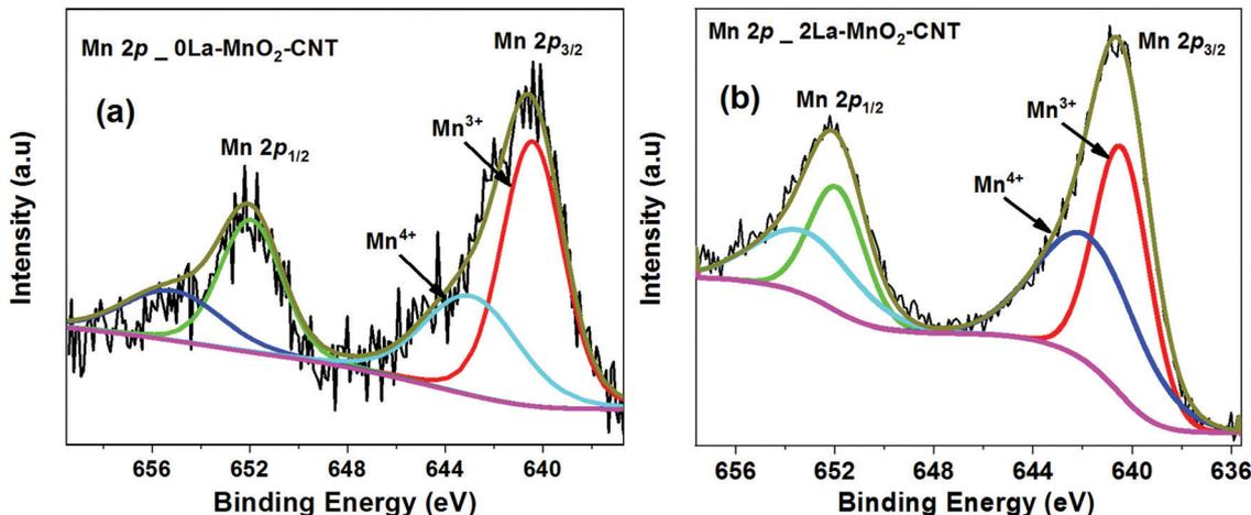
Fig. 3 XPS spectra of Mn 2p of 0La-MnO<sub>2</sub>-CNT (a) and 2La-MnO<sub>2</sub>-CNT (b).
