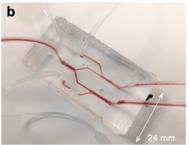
Fig. 3 Development of a novel "EDTA-quenched" device incorporating a chaotic mixer (a) schematic of the EDTA-quenched device design. A stream of high-concentration (50 mM) EDTA is introduced just after the collagen and tissue factor patch and mixed into the bloodstream using a chaotic mixer. (b) A photograph of the fabricated device.
