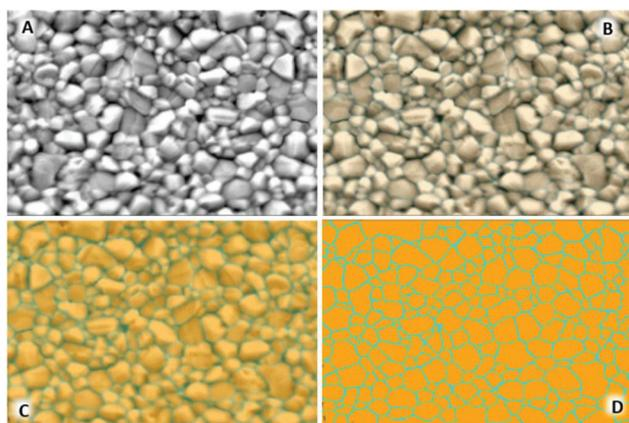
**Fig. 2** SEM of MAPbI<sub>3</sub> thin-film deposition from candidate A solvent system with 30 000× magnification (A) and the Zen Blue image analysis segmentation (B–D). (A) Mirrored image of the base data for the image analysis software to segment. To illustrate the accuracy of the segmentation the label opacity is increased (B–D) with the final result (D) typical of the segmented data analysed to extrapolate crystal size characteristics.
