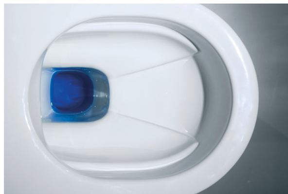
Fig. 3 The urine-separating toilet safe! from LAUFEN, implementing the urine trap. The special structures at the front-end of the toilet direct the urine towards the (nearly invisible) urine trap.<sup>112</sup> Copyright LAUFEN.<sup>123</sup>
