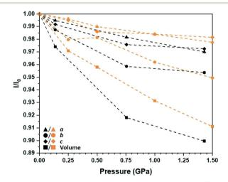
Fig. 5 Compression curves for the unit cell parameters of [Pt(bqddibutyl)2] up to 1.50 GPa, as fraction of those recorded at ambientpressure, determined from experiment (black) and a simulated pressure series using the CASTEP simulation package (orange). Error bars on the experimental data points are smaller than symbols used.
