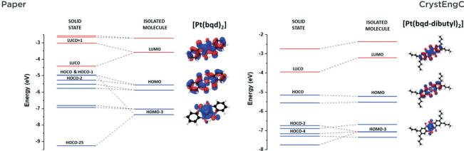
Fig. 3 Construction of crystalline orbitals (COs) from molecular orbitals for [Pt(bqd)<sub>2</sub>], as previously published,<sup>24</sup> and [Pt(bqd-dibutyl)<sub>2</sub>], as defined at the gamma point. Blue and red lines indicate occupied and unoccupied orbitals respectively. The COs from HOCO-7 to HOCO-24 inclusive for [Pt(bqd)<sub>2</sub>] have been removed for simplicity.
