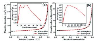
Fig. 9  $N_2$  adsorption–desorption isotherms and corresponding pore size distributions (inset) of (a) the  $Cu_2O$  hollow spheres and (b)  $Cu_2O$  nanocages.
