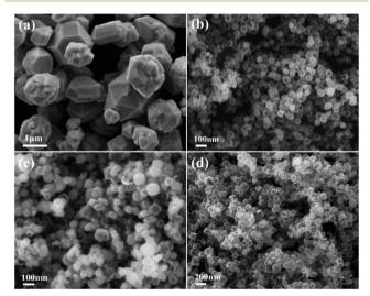
Fig. 4 SEM images of the Cu<sub>2</sub>O morphology synthesized under different reaction conditions: 0 g NH<sub>4</sub>NO<sub>3</sub> (a) and (b) 0.18 g NH<sub>4</sub>NO<sub>3</sub> were added at 50 °C; the reaction temperature was 35 °C (c) and 65 °C (d) with 0.12 g NH<sub>4</sub>NO<sub>3</sub>.
