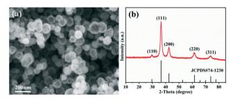
Fig. 1 (a) The SEM image and (b) XRD pattern of the synthetized Cu<sub>2</sub>O hollow spheres.
