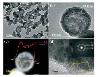
Fig. 2 (a) Low magnification TEM image of the Cu<sub>2</sub>O hollow spheres; (b) TEM image of a single Cu<sub>2</sub>O hollow sphere; (c) corresponding EDX line scan; (d) HRTEM image (inset: SAED image).
