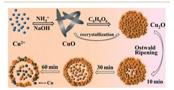
Fig. 5 Schematic diagram of the formation process of Cu<sub>2</sub>O hollow spheres.
