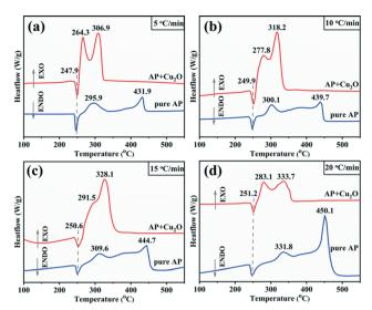
Fig. 7 DSC thermographs of AP and the mixture of AP with  $Cu_2O$  at different heating rates: (a) 5 °C min<sup>-1</sup>; (b) 10 °C min<sup>-1</sup>; (c) 15 °C min<sup>-1</sup>; (d) 20 °C min<sup>-1</sup>.
