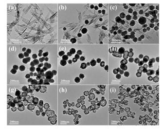
Fig. 3 TEM images of the samples with different reaction times: (a) after 5 min of adding NaOH; (b) after adding AA and reacting for 10 s; (c) 1 min; (d) 5 min; (e) 10 min; (f) 20 min; (g) 30 min; (h) 60 min; (i) 120 min.
