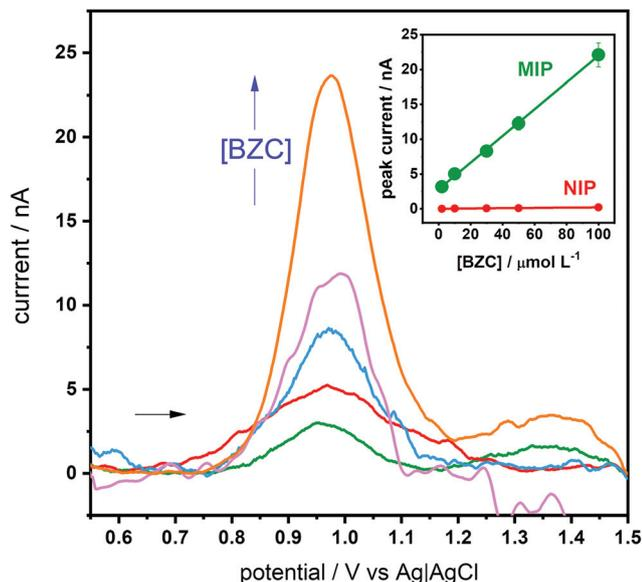
Fig. 4 SWVs of BZC in PBS (2, 10, 30, 50 and 100  $\mu\text{mol L}^{-1}$ ), detected using the optimized GCE-MIP sensing device (potential range from +0.5 to +1.5 V, at a frequency of 25 Hz, pulse amplitude of 20 mV and step potential of 2.5 mV, baseline correction with moving average level 2). Inlay: the corresponding calibration curve and the calibration curve for the NIP.
