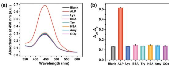
Fig. 3 (a) Typical absorption spectra and (b) the relative change of the absorption of OPDox catalyzed by  $2.5~\mu g~mL^{-1}$  of the 2D-MOF with  $2~\mu M$  of PPi in the absence and presence of 20 U  $L^{-1}$  of ALP, and 20 nM of Lys, BSA, Try, HSA, Amylase, and GOx.  $A_{20}$  and  $A_{0}$  were the absorption of OPDox at 450 nm at 0 min and 20 min, respectively. Each error bar shows the standard deviation of three independent measurements
