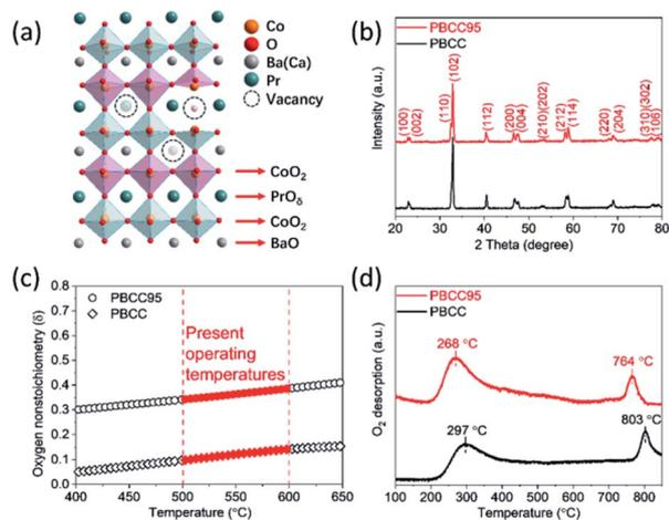
**Fig. 1** Material characterization of PBCC and PBCC95 electrodes. (a) Schematic of the crystal structure for the PBCC double perovskite with A-site deficiency; (b) XRD patterns of PBCC and PBCC95; (c) the oxygen non-stoichiometry of PBCC and PBCC95 at temperatures between 400 and 650 °C; and (d) O<sub>2</sub>-TPD profiles of PBCC and PBCC95.
