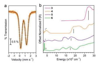
Fig. 3 (a)  $^{57}$ Fe Mössbauer spectra for a powder sample of 4 collected at 80 K. Open circles represent the experimental data, and the black line represents the fit to the spectrum. (b) Diffuse reflectance of 3–6 measured in KBr at room temperature where the black bars mark the MMCTs. The asterisks mark absorbances from the ligand, and the water absorbance at  $\sim$ 3300 cm $^{-1}$  has been manually removed from the data.
