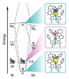
Fig. 6 Qualitative molecular orbital diagram depicting the natural orbitals of the  $\sigma\text{-bonding}$  and -antibonding orbitals and the orbital with primarily  $3d_z^2$  orbital character for compound 3.
