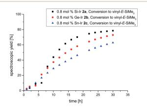
Fig. 5 Plot of the spectroscopically determined conversion to E-vinyltrimethylsilane 60 °C using the 0.8 mol% catalyst. Black = Si-Ir 2a, red = Ge-Ir 2b, blue = Sn-Ir 2c.
