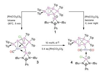
Scheme 2 Synthesis of  $Si_7$  rhodium complexes 3 and 4 from silylene-functionalized  $Si_6$  siliconoid 1.
