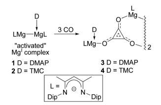
Scheme 1 Previously reported syntheses of magnesium deltate complexes,  ${\bf 3}$  and  ${\bf 4}$  (Dip = 2,6-diisopropylphenyl, DMAP = 4-dimethylaminopyridine,  $TMC = :C\{(MeNCMe)_2\}).$
