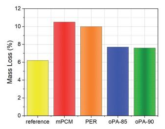
Fig. 6 Noncombustibility tests of concrete samples.
