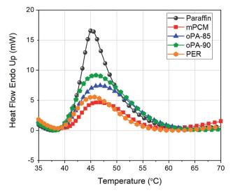
Fig. 1 DTA curves of microcapsules.
