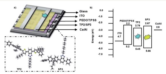
Fig. 3 (a) 3D Schematic structure of the devices and 3D chemical structures of SP3 and TP2, (b) energy diagram of layers deposited for the OLED devices.
