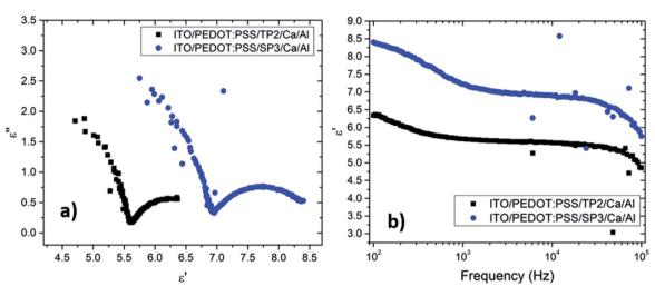
Fig. 5 (a) Cole-Cole plots of impedance for fabricated OLED device with TP2 and SP3 films. (b) Variation of real part of dielectric constant depend on frequency for fabricated OLED device with TP2 and SP3.
