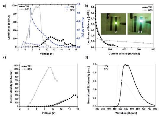
Fig. 4 (a) Luminance-voltage, EQE-voltage, (b) luminous (current) efficiency-voltage and inlet presented the light emission of OLEDs with an emissive layer SP3 and TP2 polymers, (c) current density-voltage, (d) normalized EL intensity characteristics.
