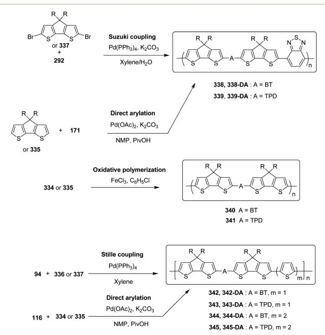
Scheme 96 Synthesis of polymers 338, 338-DA, 339, 339-DA, 340-342, 342-DA, 343, 343-DA, 344, 344-DA, 345 and 345-DA, using Suzuki, Stille, oxidative and direct arylation polymerization techniques.
