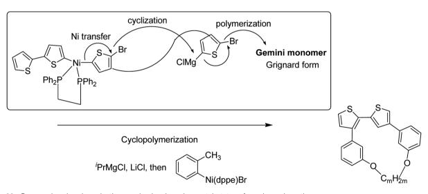
Scheme 20 Proposed cyclopolymerization mechanism based on catalyst-transfer polycondensation.
