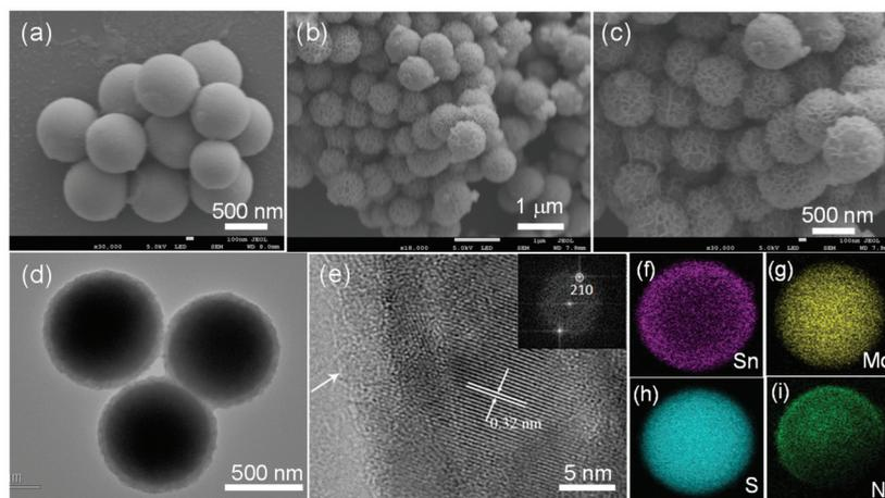
**Fig. 4** (a) SEM image of the MoG nanospheres; (b and c) SEM images of the MoS<sub>2</sub>@SnS heterostructures with different magnifications; (d) TEM image of the MoS<sub>2</sub>@SnS heterostructures; (e) HRTEM image of the MoS<sub>2</sub>@SnS heterostructures with the corresponding fast Fourier transform (FFT) pattern (inset); EDS elemental mapping of (f) Sn, (g) Mo, (h) S and (i) N elements in the MoS<sub>2</sub>@SnS composite.
