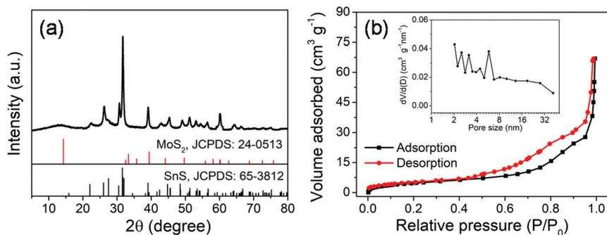
Fig. 2 (a) XRD pattern and (b) N<sub>2</sub> adsorption/desorption isotherms and pore size distribution curve (inset) of the MoS<sub>2</sub>@SnS heterostructure.
