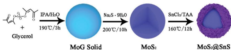
Fig. 1 Schematic illustration of the synthesis of MoS<sub>2</sub>@SnS heterostructure.
