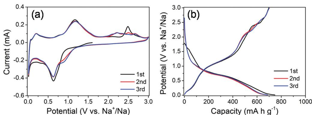
**Fig. 5** (a) CV curves of the MoS<sub>2</sub>@SnS heterostructure at a scan rate of 0.1 mV s<sup>-1</sup> and (b) galvanostatic charge/discharge profiles of the MoS<sub>2</sub>@SnS heterostructure at a current density of 0.1 A g<sup>-1</sup>.
