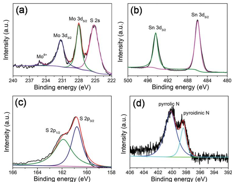
Fig. 3 High-resolution XPS spectra of the MoS<sub>2</sub>@SnS heterostructure. (a) Mo 3d; (b) Sn 3d; (c) S 2p; and (d) N 1s spectra.
