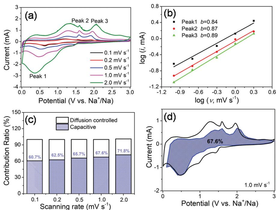
Fig. 7 (a) CV curves at various scan rates ranging from 0.1 to  $2.0 \text{ mV s}^{-1}$ ; (b) plots of  $\log(i)$  vs.  $\log(v)$  at the sharp cathodic/anodic peak pair (peak current:  $i$ , scanning rate:  $v$ ); (c) capacity contributions at different scan rates; and (d) capacitive charge storage contribution at a scan rate of  $1.0 \text{ mV s}^{-1}$ . The estimated pseudocapacitance contribution is shown in the blue region.
