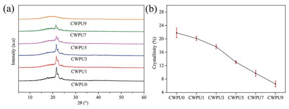
Fig. 6 XRD spectra (a) and crystallinity (b) of CWPU membranes.
