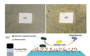
Fig. 12 (a) and (b) Show the text results of the CWPU7 membrane in E. coli and Staphylococcus aureus. (c) Shows the process of the antibacterial CWPU film.
