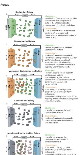
Fig. 3 Schematic working principle of sodium-ion (a), magnesium-ion (b), magnesium-sodium dual-ion (c), aluminum-ion (d), and aluminumgraphite dual-ion (e) batteries and the respective advantages and disadvantages of each system.
