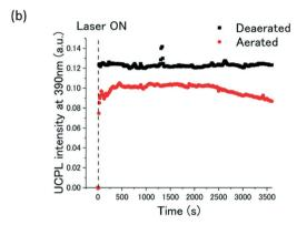
Fig. 4 (a) PL spectra of A1-Firpic-Dec in deaerated (black) and aerated (red) water under 445 nm excitation ([A1] = 10 mM, [Flrpic] = 100  $\mu$ M, [Dec] = 80 mM). Scattered excitation laser light was removed using 400 and 425 nm short-pass filters. (b) Time dependence of the UCPL intensity of A1-Firpic-Dec in deaerated (black) and aerated (red) water at 390 nm.
