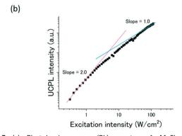
Fig. 3 (a) Photoluminescence (PL) spectra of A1-FIrpic-Dec in deaerated water ([A1] = 10 mM, [Firpic] = 100  $\mu$ M, [Dec] = 80 mM,  $\lambda_{ex}$  = 445 nm). Scattered excitation laser light was removed using 400 and 425 nm short-pass filters. (b) Excitation intensity dependence of the UCPL intensity of A1-Firpic-Dec in deaerated water at 390 nm. The red and blue lines are the fitting results with slopes 2.0 and 1.0, respectively.
