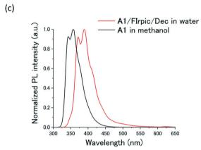
Fig. 2 (a) Photographs of Dec ([Dec] = 80 mM), A1-Firpic-Dec ([A1] = 10 mM, [Flrpic] = 100  $\mu$ M, [Dec] = 80 mM), and A1 ([A1] = 10 mM) in water. (b) DLS profile of A1-FIrpic-Dec in water ([A1] = 10 mM, [FIrpic] = 100  $\mu$ M, [Dec] = 80 mM). (c) Fluorescence spectra of A1 in methanol (black, [A1] = 0.25 mM,  $\lambda_{ex}$  = 241 nm) and A1-Firpic-Dec in water (red, [A1] = 10 mM, [Firpic] = 100  $\mu$ M, [Dec] = 80 mM,  $\lambda_{ex}$  = 280 nm).
