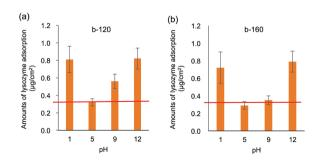
Fig. 6 Lysozyme adsorption results on (a) b-120 and (b) b-160 after treatment at pH 1, 5, 9, and 12. Red line shows adsorption without pH treatment.
