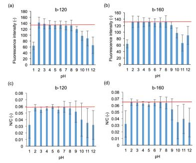
Fig. 5 Results of fluorescence intensity of rhodamine 6G on (a) b-120 and (b) b-160 after pH treatment. Red line shows fluorescence without pH treatment. Results of N/C calculation from XPS measurement on (c) b-120 and (d) b-160 surfaces after pH treatment. Red line shows N/C without pH treatment.
