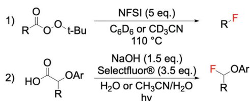
Scheme 4 Examples of radical fluorinations using electrophilic fluorinating agents containing N–F bonds: (1) fluorination of tert -butyl peresters to form \text{C}(\text{sp}^3)\text{-F} bonds, 65 and (2) photo-decarboxylative fluorination of 2-aryloxy and 2-aryl carboxylic acids. 67
