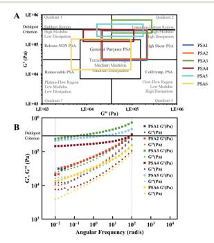
**Fig. 3** (A) Chang's viscoelastic window of pressure-sensitive adhesives applied to the synthesised PSAs and (B) frequency sweep measurements performed at room temperature by rheology.
