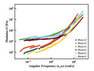
Fig. 4 Rheological master curves of G' obtained for the different PSA formulations using the time–temperature superposition principle ( $T_{ref} = 25 \, ^{\circ}\text{C}$ )
