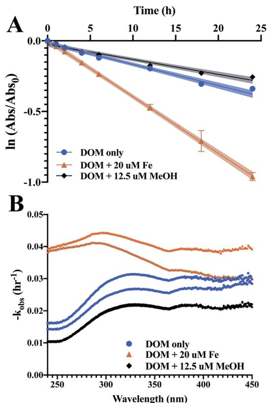
Fig. 3 Absorbance loss of 10 mg C L<sup>-1</sup> GSL summer DOM isolate and amended solutions over 24 h irradiation. (A) Log linearised pseudo first-order kinetics of absorbance loss at 254 nm. (B) Fitted observed pseudo first order rates of absorbance loss across wavelengths.
