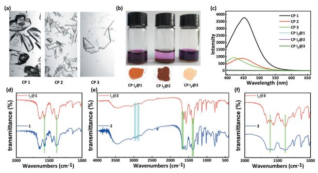
Fig. 5 (a) Photographic images of CPs 1 (left), 2 (middle), and 3 (right). (b) Photographs of I<sub>2</sub> adsorption in solutions and crystalline I<sub>2</sub> inclusion compounds of CPs 1 (left), 2 (middle), 3 (right). (c) Solid luminescence spectra of CPs 1-3 before and after I2 adsorption in cyclohexane solution of  $l_2$  for 48 h. IR spectra of CPs (d) 1, (e) 2, (f) 3 before and after  $l_2$  adsorption in cyclohexane solution of  $l_2$  for 48 h.
