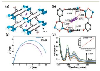
Fig. 6 (a) I<sub>2</sub> guest molecules are encapsulated in the channels in CP  $I_2@2$ . (b) The linkages between  $I_2$  and the framework through C= $O\cdots I$ and  $\pi \cdots I$  interactions (green dashed line –  $\pi \cdots I$  interaction; red dashed line - C=O···I interaction). (c) Electrochemical impedance spectra of CP 2 and CP I2@2. (d) The I2 release process of CP I2@2. The inset of figure is the kinetic study of I2 release over time.
