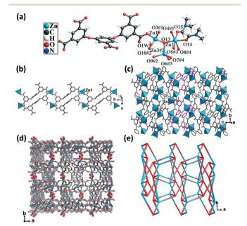
Fig. 3 (a) Coordination environment of the Zn(II) atoms in CP 3. Color code: Sky blue - Zn; red - O; gray - C. (b) The 1D chain formed by the Zn1 atoms and  $L^{5-}$  ligands. (c) The 2D layer formed by the Zn2 atoms and 1D chains. (d) 3D framework. (e) The topological network with the point symbol  $(4^5 \cdot 6^5)$ .
