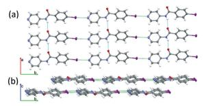
Fig. 3 INPBA structure: (a) 2D sheets formed by  $N_{pyr}\cdots I$  halogen bonding in green and perpendicular  $N-H\cdots O=C$  carboxamide hydrogen bonds in blue; (b) isolated layers. Thermal ellipsoids are drawn at the 50% probability level.
