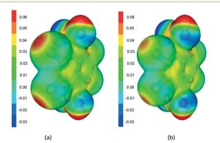
Fig. 4 Electrostatic potentials plotted at the outer contour of an electron density of 0.004 a.u. and values vary from -0.03 to 0.06 a.u for H<sub>2</sub>Br<sub>4</sub>BDC (a) and H<sub>2</sub>Cl<sub>4</sub>BDC (b). All calculations were performed at the  $\omega$ B97X-D/def2-TZVPP level of theory.
