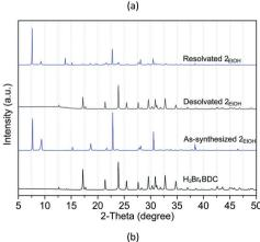
Fig. 5 TG curves of H<sub>2</sub>Br<sub>4</sub>BDC and all the solvates (a) and PXRD patterns (bottom to top) of H<sub>2</sub>Br4BDC, as synthesized 2<sub>EtOH</sub>, desolvated  $2_{EtOH}$ , and resolvated  $2_{EtOH}$  (b).
