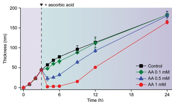
Fig. 4 Graphs of film thickness versus reaction time in the IGI-based solution ( $[\text{Fe}^{2+}] = 10 \text{ mM}$ ,  $[\text{TA}] = 1 \text{ mM}$ ). AA (0.1, 0.5, or 1 mM) was added to the solution after 3 h of reaction.
