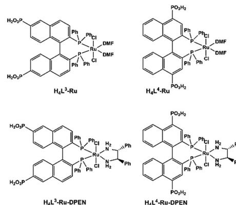
Scheme 10 Molecular structures of Ru-L<sup>4</sup> complexes of binaphthalene-bisphosphonic acids. Reprinted with permission from ref. 10f. Copyright 2020, Springer Nature.
