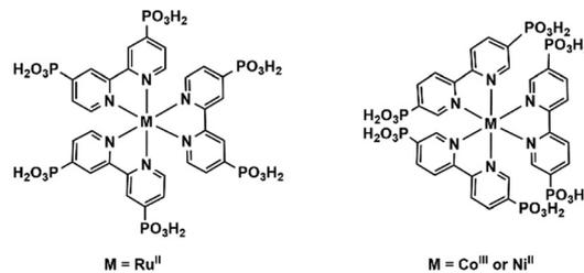
Scheme 8 Molecular structures of metalloligands Ru<sup>II</sup>(4,4'-dpbpyH<sub>4</sub>)<sub>3</sub><sup>2+</sup> and [M(5,5'-diphosphonic acid)<sub>3</sub>]<sup>n+</sup>.
